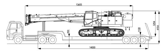
■ Transportation mode II: dismantle the counterweight, jib and lifting hook, transport through two vehicles with maximum weight of single piece transportation 34t, 13.7m x 2.99m x 3.25m (L x W x H)
