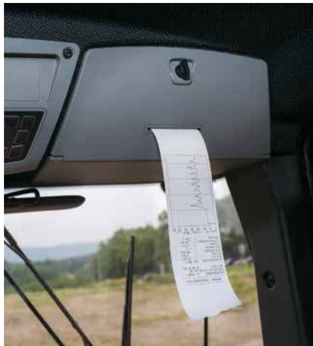
Integrated printer: for documentation of compaction results.
