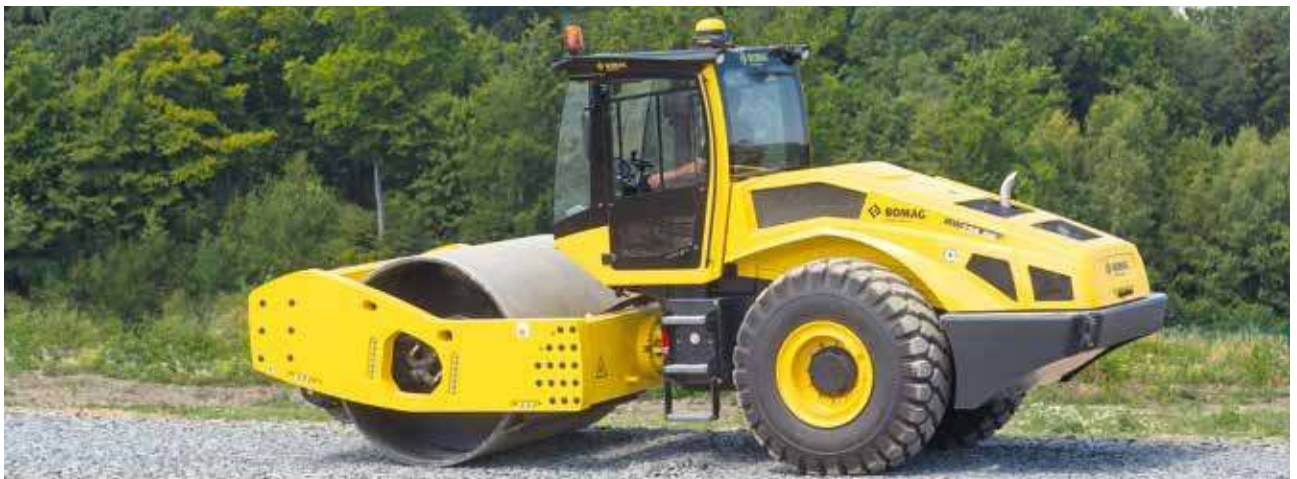
Knowing what's going on: continuous dynamic compaction control, layer for layer, across the entire construction site.
