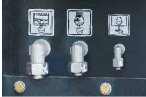
Smart: operating materials can be drained externally.
