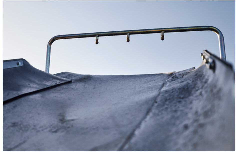
Water spraying system for efficient dust suppression, pump included.
