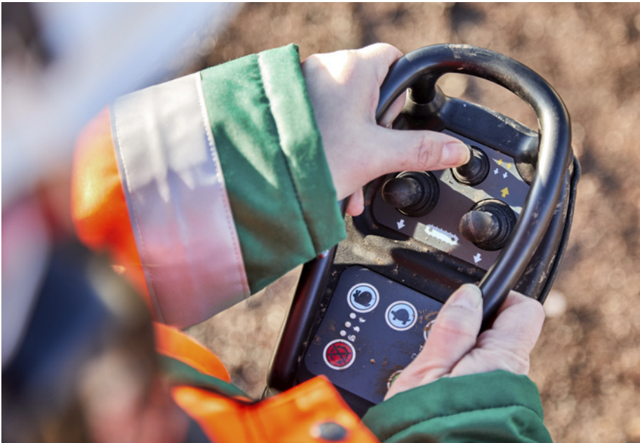
Remote controller for crawler tracks as standard.
