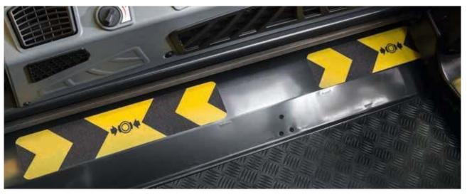
Conventional pedals are no longer included, increasing both the viewing scope for the driver and the movability of his seat.
