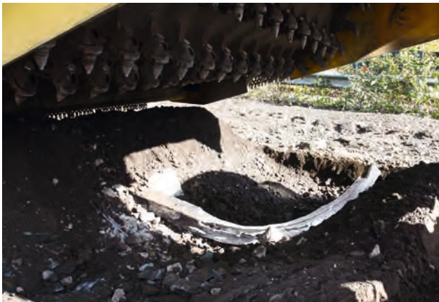
The hydraulic overload protection system prevents unwanted surprises.
