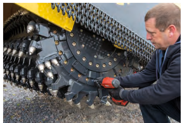
Changing the edge segments without having to remove the rotor.
