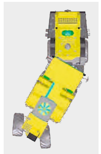
Asynchronous steering. (Crabwalk)
