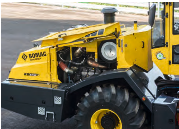
All service points are easy to access: water filter, AdBlue, and the central lubrication system.
