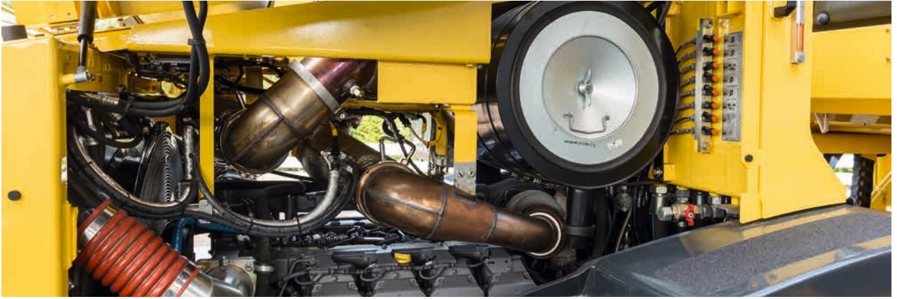
TIER 4 final with dual SCR system.
