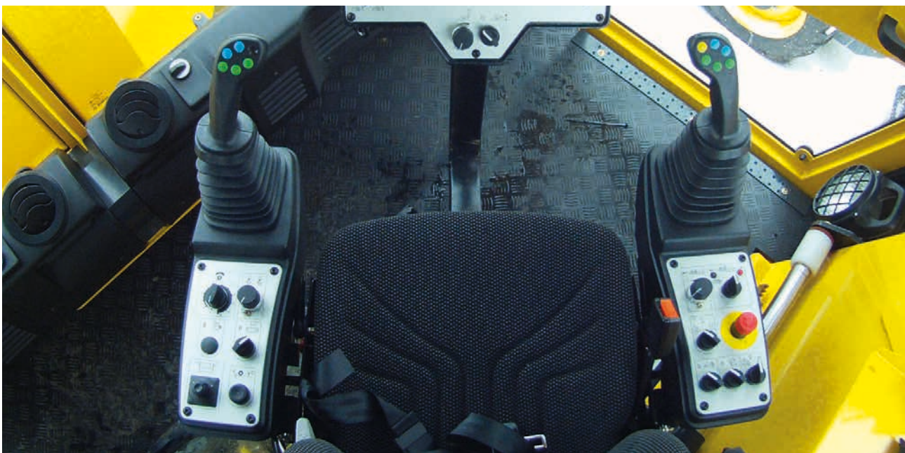
Two joysticks on the arm rests for easy handling of the machine.
