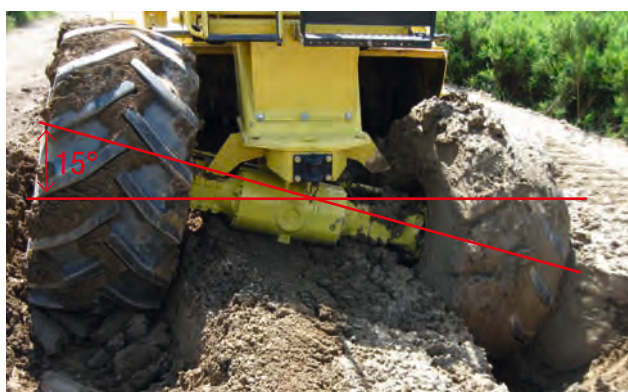
Non-spin oscillating axle +/- 15°.
