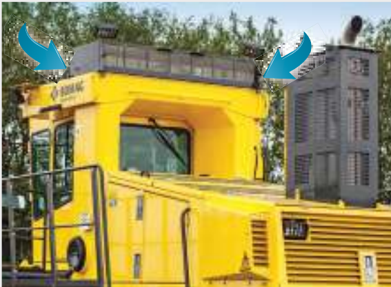
High level suction for cooling and combustion air with minimum dust levels.
