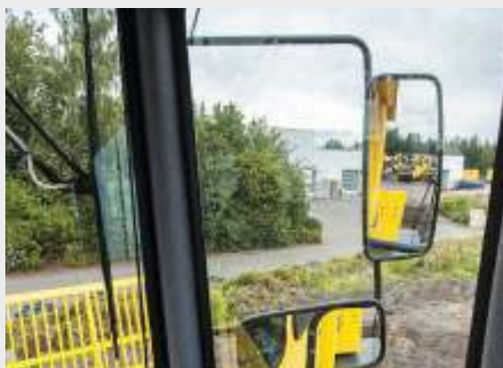
Large mirrors on both sides combined with large glass areas for excellent all-round visibility.
