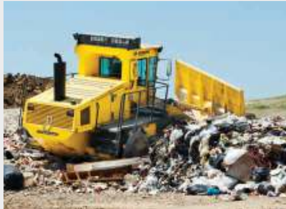
Optimum compaction is achieved by the effect of the oscillating joint, which supplies uniform load distribution to the compactor wheels.
