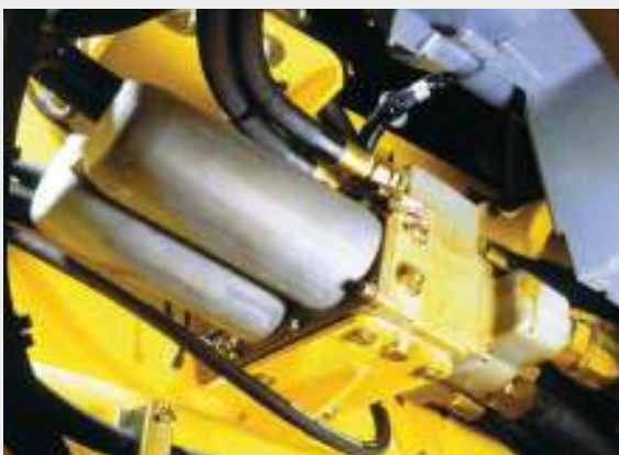
Electronic monitoring of hydraulics return filter system.
