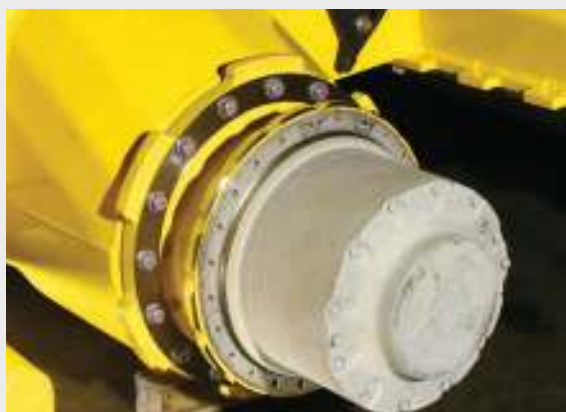
Two independent braking systems (hydrostatics for the service brake, multiple discs for the parking brake).
