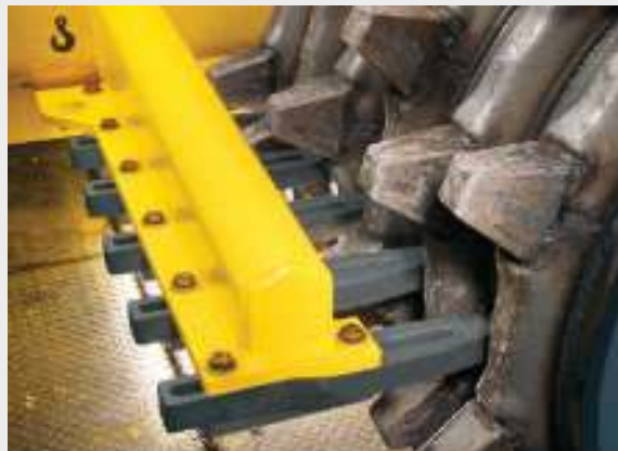
Clean wheels with effective scrapers (optimum compaction).
