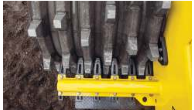
Adjustable scraper for uninterrupted operation.
