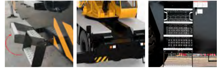
Extra-wide aluminum alloy access deck and ladder Rotatable footstep.
