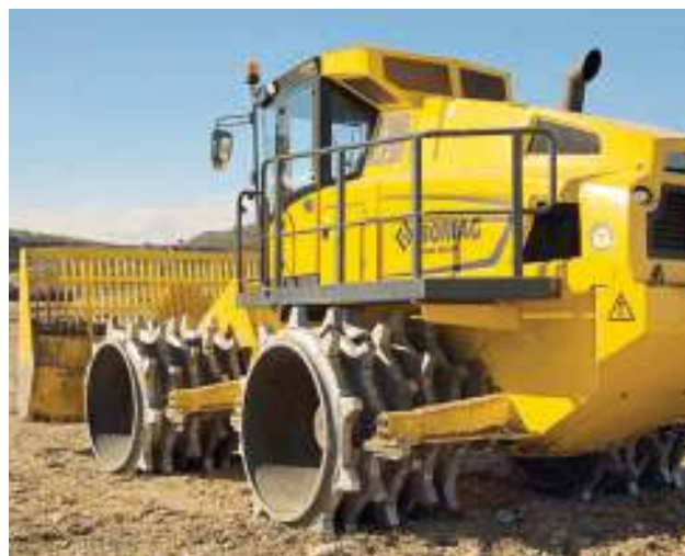
The service platform gives access to the maintenance area.
