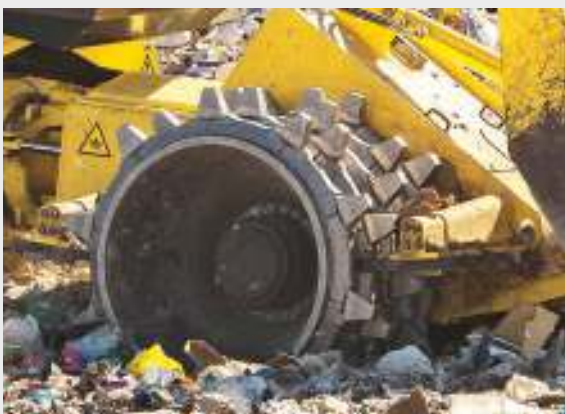
Scrapers guarantee clean wheels and high compaction.
