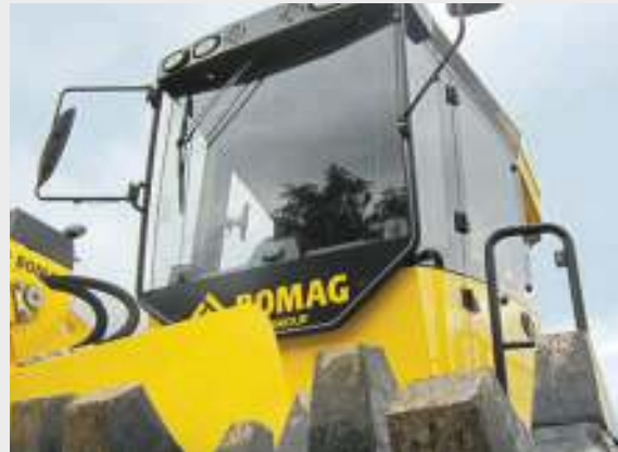
Cab design complies with ROPS and FOPS regulations.
