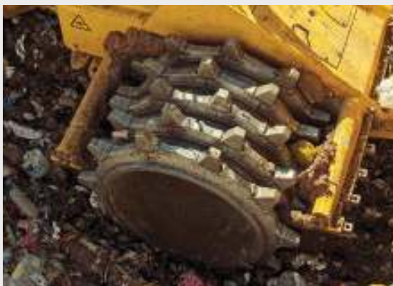
Clean wheels with effective scrapers (optimum compaction).
