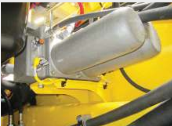
Electronic monitoring of hydraulics return filter system.
