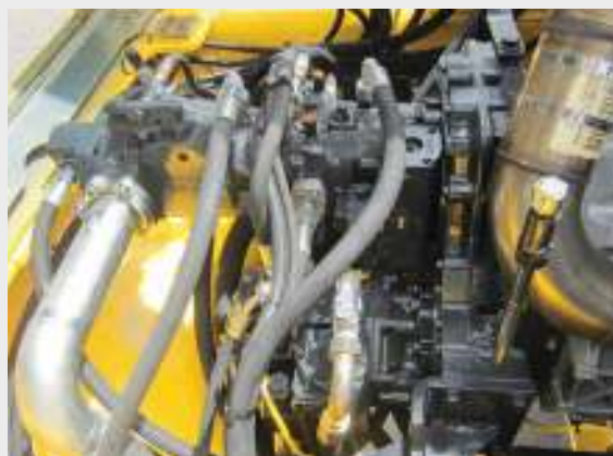
Hydraulic wheel drive with „load limit control“ (load-related speed control) (BC 473).
