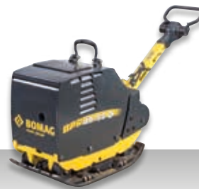
BPR 45/55 D Operating weight: 400 kg Centrifugal force: 45 kN Working width: 550 mm
