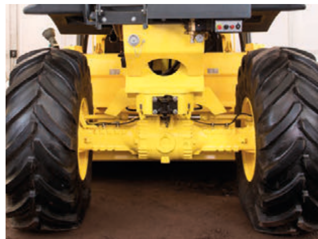
Non-spin oscillating axle \pm 15^\circ (RS 460).
