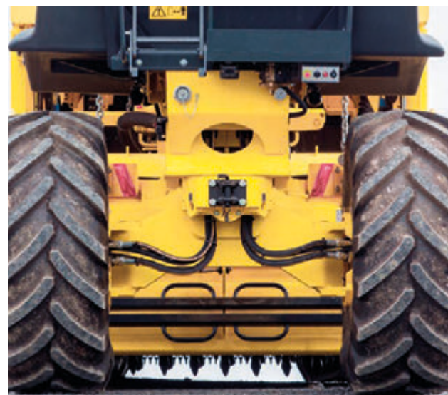
Rear axle with powerful single drives (RS 500).
