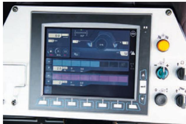
The screen displays and sets the metering systems.
