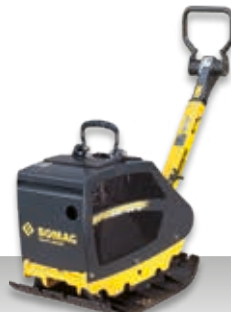
BPR 40/60 D Operating weight: 260 kg Centrifugal force: 40 kN Working width: 600 mm
