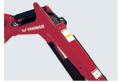
The boom hose and cylinder are covered for protection.
