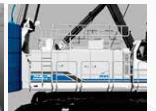
Catwalk with handrails and folding type upper house handrails
