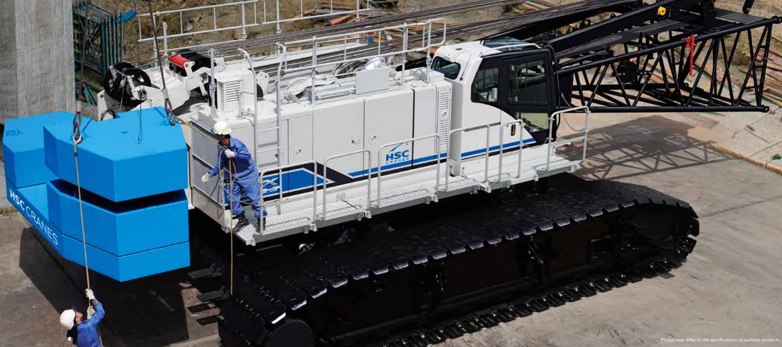
Counter weights and boom can be transported together
