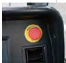
▲ Emergency engine stop switch (for crane operation)
